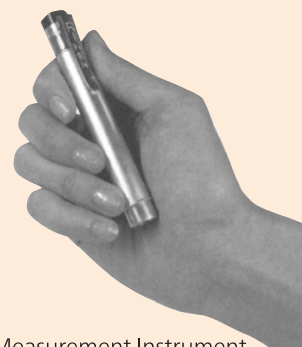
Radiation Measurement Instrument Pocket Dosimeter
