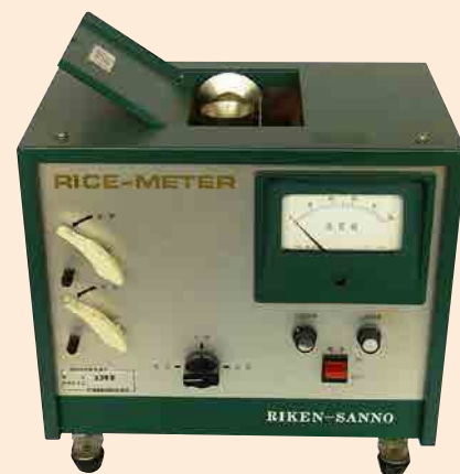
Brown Rice Quality Measuring Device "Rice Meter"
