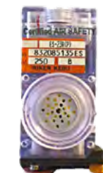
The potentiostatic electrolysis method sensor "ES-23 series" contributed to commercialization of gas detectors for semiconductor plants.
