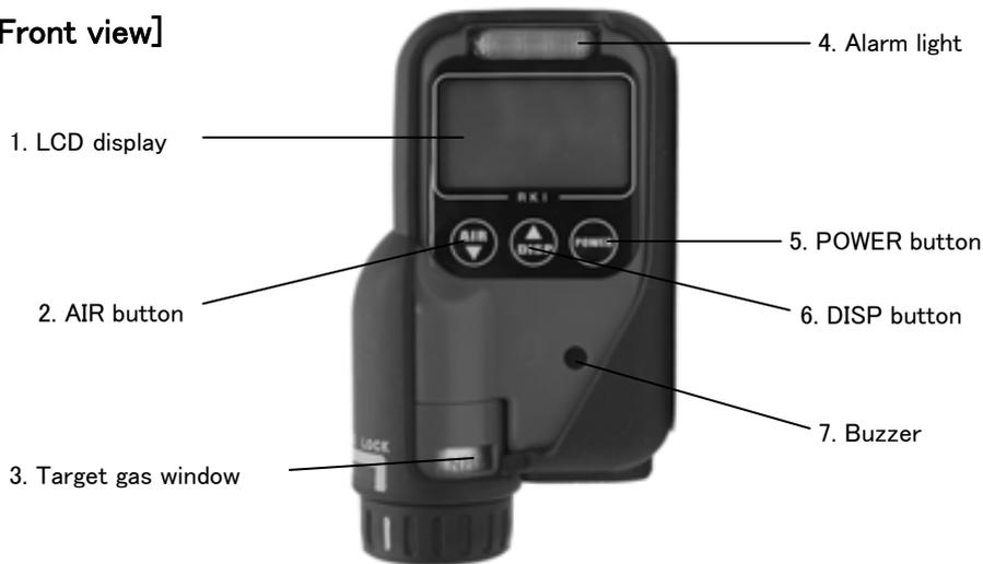
1. LCD display : Indicates gas detection results and various information.
