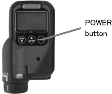
In any mode, the power is turned off by pressing and holding the POWER button for about 3 seconds.
